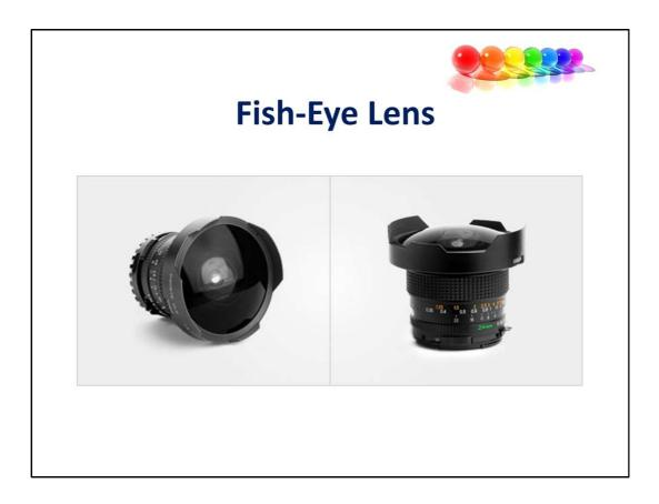
A fisheye lens is a specialized, wide-angle lens that provides extremely wide images by changing straight lines into curves. It can sometimes produce circular, convex, or oval images by distorting the perspective and creating a 180° image. The range of focal length varies between 7~16mm in a fish-eye lens.
