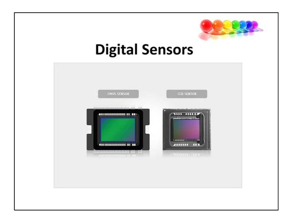
An **image sensor** is a device that converts an optical image into an electronic signal. It is used mostly in digital cameras, camera modules and other imaging devices. Early analog sensors were video camera tubes, most currently used are digital **charge-coupled device** (CCD) or **complementary metal–oxide–semiconductor** (CMOS) **active pixel sensors**.
