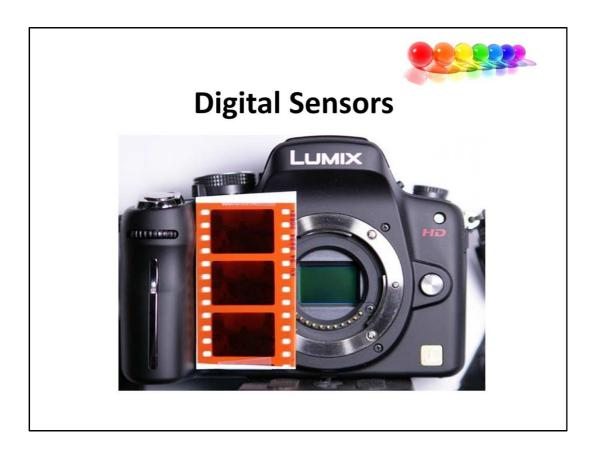
An **image sensor** is a device that converts an optical image into an electronic signal. It is used mostly in digital cameras, camera modules and other imaging devices. Early analog sensors were video camera tubes, most currently used are digital **charge-coupled device** (CCD) or **complementary metal–oxide–semiconductor** (CMOS) **active pixel sensors**.
