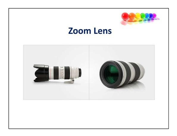
Zoom lenses have variable focal lengths, and are extremely useful. Some can range between a wide-angle and a telephoto (i.e. 24 to 300mm) so you have extensive versatility for composition. The trade off with zoom lenses is the aperture. Because of the number of elements required in constructing these lenses, they have a limited ability to open up and allow in light. So unless you're prepared to outlay a lot of money, you will give up lens speed.
