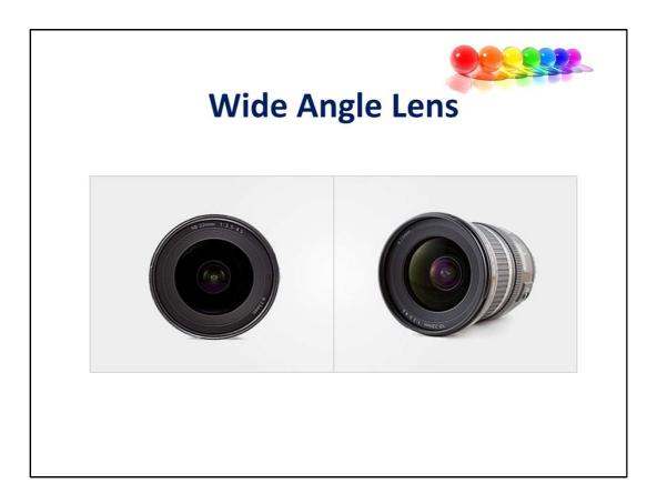
A wide-angle has a shorter focal length (10 thru 42mm) when compared to a standard lens. This enables you to capture a comparatively wider angle of view. A wide-angle lens is a natural choice for capturing outdoor landscapes and group portraits. In fact, wide angle can be the only way to capture the complete setting without omitting any important elements in the image. In this manner, you can use wide-angle lenses to capture a deep DOF.
